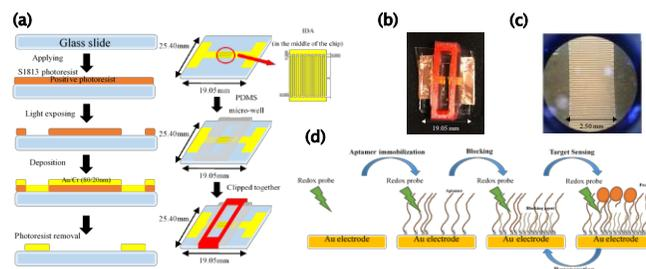
Figure 1. IDA chip (a)device setup, (b)top-view, and (c)under microscope. (d)Scheme of fabrication and detection on aptasensor
