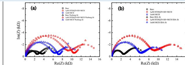
Figure 2. Nyquist plot of IDA electrode EIS raw data fitted with (a) Warburg element (b) IDA element in Randles equivalent circuit.
